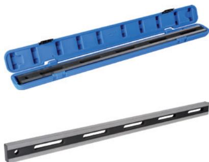
The straightedge is a measuring tool used for checking that a surface is level using the light gap method. The straightedge is used specifically to check cylinder heads when changing the cylinder head gasket. If the en-
