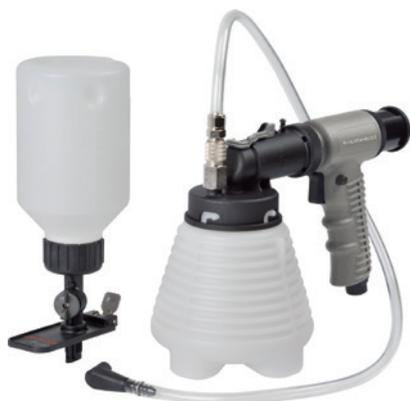
This pneumatic device is used to bleed hydraulic circuits in brake and clutch systems. The device operates according to the Venturi principle. The brake fluid is drawn off via the bleed nipple. A refiller is positioned on the expansion tank side and automatically regulates the fill level of the expansion tank.
