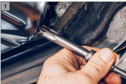
**Repair Kit, oil drain plug thread**
