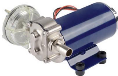
Small self-priming, electric pump with bronze gears, housing made of nickel-coated brass, spindle made of stainless steel. Partic-
