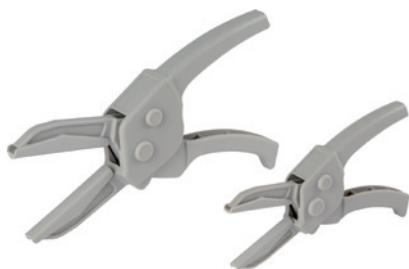
The universal locking pliers are used to disconnect various cooling water and vacuum hoses. They prevent for example cooling water from escaping or the cooling system from running empty, e.g. when water pumps, thermostats, fittings etc. are replaced. There is no longer any need for laborious ventilation of the cooling system.
