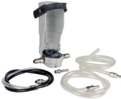
This practical hydraulic pump in a design suitable for use in workshops is used for pumping off or refilling and filling all non-easily flammable fluids, such as engine and transmission oil, radiator antifreeze, brake fluid, etc. The pump is either powered electrically, using a cordless screwdriver or alternatively also pneumatically using an air ratchet or impact wrench.
