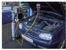
Now fill the high-pressure side of the A/C plant. Using the leak detection set extension kit, the high- and low-pressure sides can be filled simultaneously.
