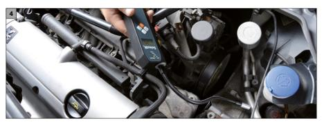
Feed the gas detector along the top of the hose connections and components at a steady speed. You can read out the respective hydrogen concentration on the display. Rising ppm values indicate a leak.
