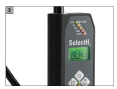
The heat-up phase is signalled by the word "HEAT" and lasts approx. 50 seconds.
