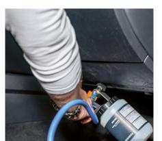
7. Now turn the device off and remove the spray pistol. Close the door and let the ventilation run for a further 2-5 minutes.
