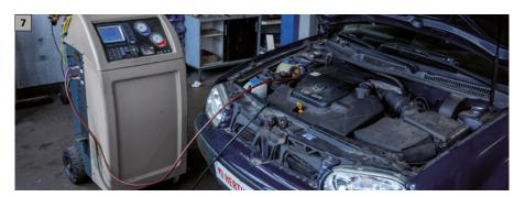
Then fill the A/C plant with the appropriate refrigerant. Finally, perform a function check.
