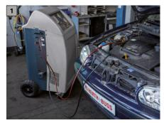
Evacuate the A/C plant using a suitable A/C service station.
