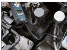
Leaks are also indicated by means of acoustic and visual signals.
