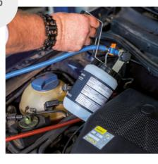
5. Open the bonnet and remove the cabin filter. Clean the pollen filter box if required and disinfect it. Set the ventilation system to level 1 and spray the disinfectant into the interior of the vehicle through the air intake opening of the HVAC system. Feed the agent in until the vehicle interior has become visibly filled with mist. Leave the mist to take effect for approx. 1 minute.
