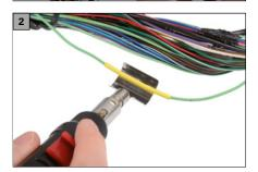
Thanks to the adjustable gas supply and the attachments included in the scope of delivery, the burner is suitable for a wide variety of operations, such as for professional heating of shrink tubing or soldering in cable lugs.
