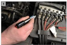
The voltage detector PlusMinus 3-28 is compatible with electronic components like engine control units, sensors etc. An earth line or -terminal is not required.
