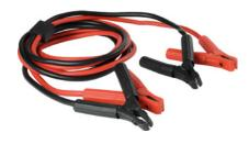
This jumper cable is made of CCA conductor material (copper coated aluminium), which offers the same conductance as a copper cable with a cross-section of 25 mm<sup>2</sup>. The professional pliers made from steel plate are reinforced
