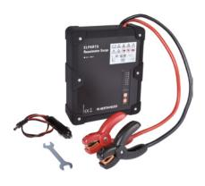
In contrast to conventional assisted start devices, this device does not have an internal battery. Very powerful capacitors instead serve as power accumulators. These can store and then dispense the power required to start the engine in a very short time. The device functions entirely off-grid and can even be charged using the residual power from the discharged
