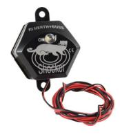
More power – More protection – More safety A sound reflection system is used for the first time in a marten repellent. This makes it possible to achieve 360° emission. A convex cone is arranged above a piezoelectric loudspeaker with a NAWI membrane. The cone has the
