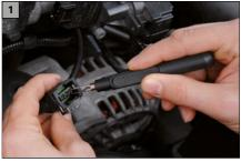
The triple set of release tools can be used to open the most common connections. The set includes three cable release tools with six blades for common crimp connectors. The tips of the tools are made from high- quality spring
