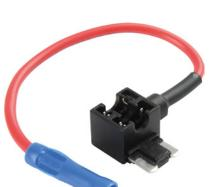
Additional loads can be connected quickly and easily using the junction bracket. The fuse previously hidden in the fuse box is removed and replaced by the additional bracket. The fuse is then placed in the bottom connection point of
