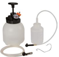
This tool is used to bleed brake or clutch hydraulics. For this purpose, the tool is connected to the hydraulic system via the compensating reservoir. The reservoir is pressurised by means of the integrated hand pump. On bleeding (on opening the bleeder nipple), the brake fluid is forced through the hydraulic pipes and replaced with an adequate
