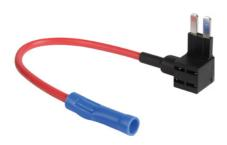
Additional loads can be connected quickly and easily using the junction bracket. The fuse previously hidden in the fuse box is removed and replaced by the additional bracket. The fuse is then placed in the bottom connection point of
