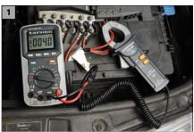
The clamp meter is suitable for measuring high flows up to 400 amperes.
