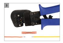
A crimp, shrink or soldered shrink connector can be used for the connection.
