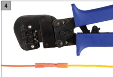
The cables are then crimped with the connector one after the other. In this example with our crimping pliers CrimPro10, alternatively with CrimPro30.
