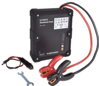
In contrast to conventional assisted start devices, this device does not have an internal battery. Very powerful capacitors instead serve as power accumulators. These can store and then dispense the power required to start the engine in a very short time. The device functions entirely off-grid and can even be charged using the residual power from the discharged
