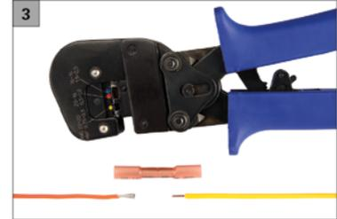
A crimp, shrink or soldered shrink connector can be used for the connection.
