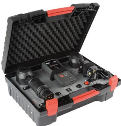
The indicator enables both the assignment of the trailer socket and the lighting function of the trailer to be checked by just one person. The tester replaces and simulates the towing vehicle or the trailer as desired. The user can have the lighting signals of the vehicle displayed on the remote control or use the remote control to activate all lights on the trailer.
