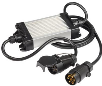
Dummy resistance load for adapting LED trailer lights on vehicles with lamp monitoring. The failure of one LED unit is detected and the load is switched off.
