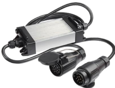
Dummy resistance load for adapting LED trailer lights on vehicles with lamp monitoring. The failure of one LED unit is detected and the load is switched off.
