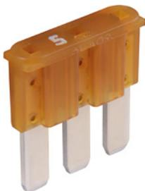
The MICRO3 fuse has three contacts, with two fuse elements sharing a common central contact. The small size means that multiple circuits can be fused in even the tightest of spaces. Very small dimensions combined with
