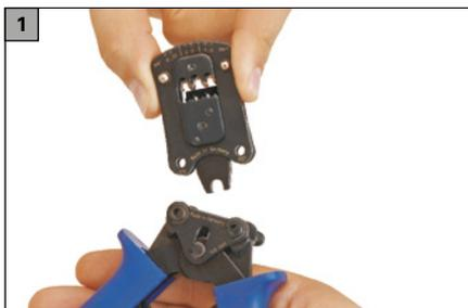
The CrimPro 10 offers a large range of processing options. Professional crimping precision for all common contacts thanks to linear die crimping. Ergonomic soft-hand grip also ensures fatigue-proof work. Inserts can be changed without additional tools.
