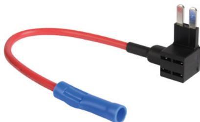
Additional loads can be connected quickly and easily using the junction bracket. The fuse previously hidden in the fuse box is removed and replaced by the additional bracket. The fuse is then placed in the bottom connection point of
