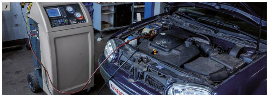
7 Then fill the A/C plant with the appropriate refrigerant. Finally, perform a function check.
