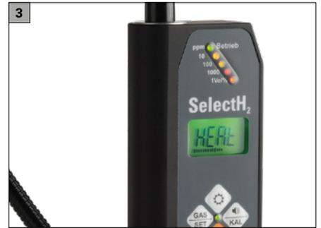
3 The heat-up phase is signalled by the word „HEAT“ and lasts approx. 50 seconds.
