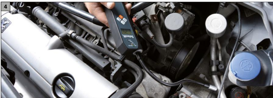
4 Feed the gas detector along the top of the hose connections and components at a steady speed. You can read out the respective hydrogen concentration on the display. Rising ppm values indicate a leak.
