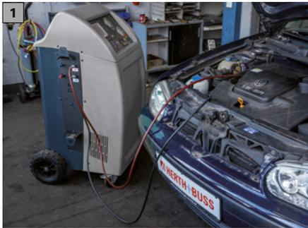
1 Evacuate the A/C plant using a suitable A/C service station.
