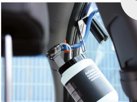
Close the doors and leave the door that the ventilation supply hose is fed through propped open in order to prevent too much of the mist from escaping. Open the compressed air supply and let the disinfectant flow in until an obvious saturation/formation of mist is visible inside the vehicle.
