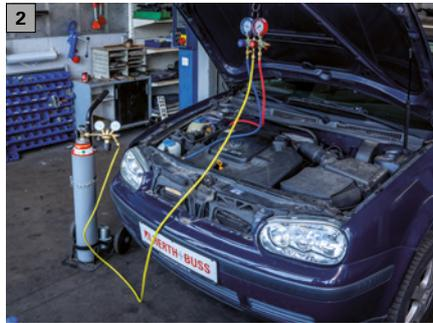
2 Now fill the high-pressure side of the A/C plant. Using the leak detection set extension kit, the high- and low-pressure sides can be filled simultaneously.
