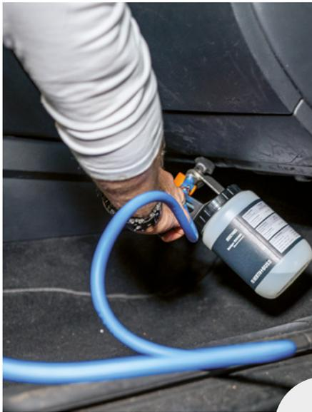
7. Now turn the device off and remove the spray pistol. Close the door and let the ventilation run for a further 2-5 minutes.
